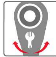
Reversible switch enables ratchet handle to move in either direction.
