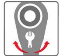
Reversible switch enables ratchet handle to move in either direction.
