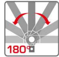
Flexible drive tilts 180° at any interval with continuous drive tension.
