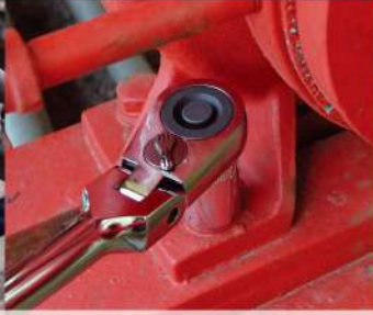
Ratchet head allows ratchet handle to travel without removing from fastener.
