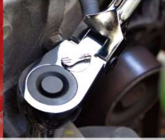
Reversible switch enables ratchet to move in either direction.
