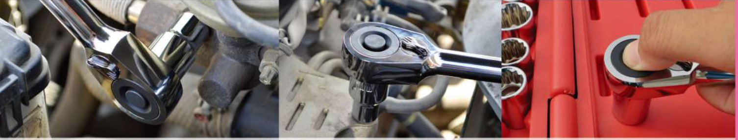
Ratchet head allows ratchet handle to travel without removing from fastener.
