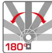
Flexible drive tilts 180° at any interval with continuous drive tension.
