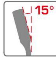
15° offset box end for knuckle clearance.
