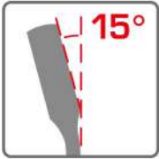
15° offset box end for knuckle clearance.
