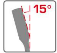
15° offset flare nut drive for knuckle clearance.
