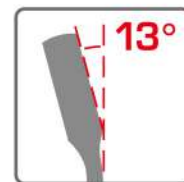
13° offset flare nut drive for knuckle clearance.
