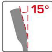
15° offset box end for knuckle clearance.
