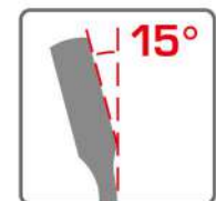
15° offset box end for knuckle clearance.
