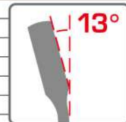
13° offset box end for knuckle clearance.
