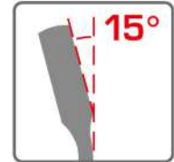
15° offset box end for knuckle clearance.
