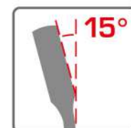
15° offset box end for knuckle clearance.
