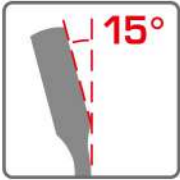
15° offset box end for knuckle clearance.
