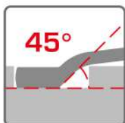
45° offset box end for knuckle clearance.
