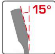
15° offset box end for knuckle clearance.
