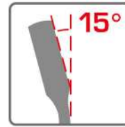
15° offset box end for knuckle clearance.
