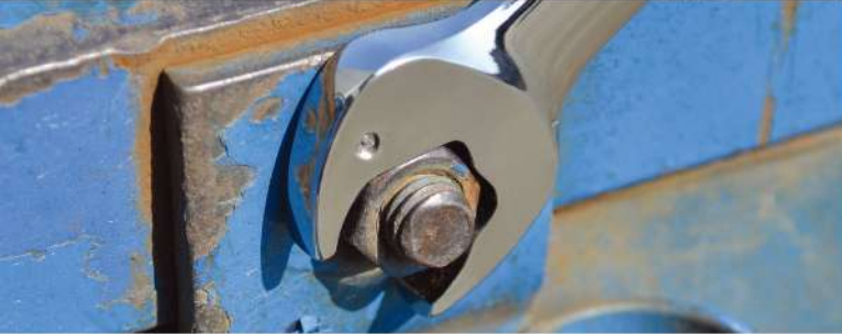
Ratchet open end allows wrench to travel without removing from fastener.
