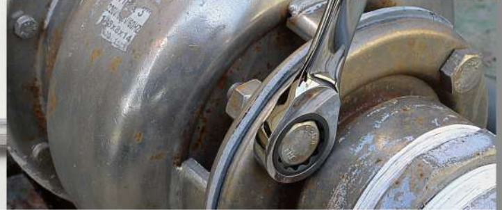
Ratchet head allows wrench to travel without removing from fastener.
