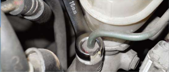
Designed to work on a variety of fittings, such as fuel, brake, and air conditioning lines.
