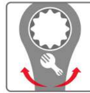
Reversible switch enables wrench to move in either direction.
