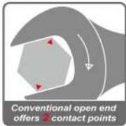
Specially designed open end gets better nut friction and minimizes slipperiness.
