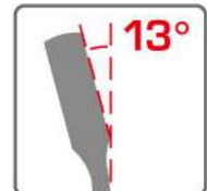
13° offset flare nut drive for knuckle clearance.
