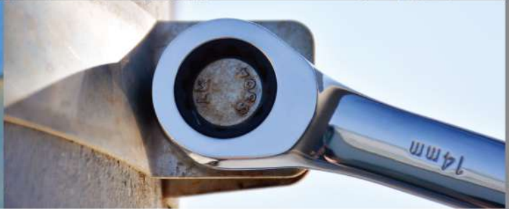
Ratchet head allows wrench to travel without removing from fastener.
