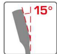
15° offset ratchet head for knuckle clearance.
