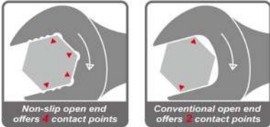
Specially designed open end gets better nut friction and minimizes slipperiness.
