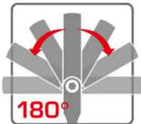
Flexible head tilts 180° at any interval with continuous head tension.
