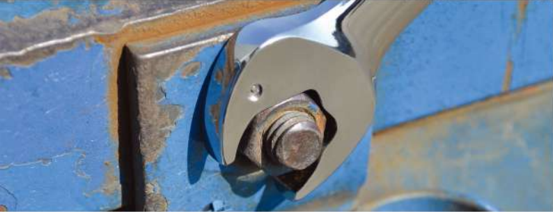
Ratchet open end allows wrench to travel without removing from fastener.
