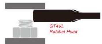
TURN RATCHET Ratchet head allows wrench to travel without removing from fastener.
