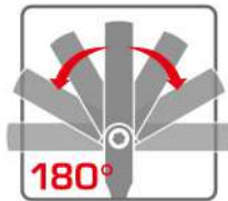
Flexible head tilts 180° at any interval with continuous head tension.
