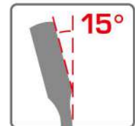
15° offset box end for knuckle clearance.
