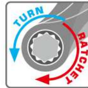
Ratchet head allows wrench to travel without removing from fastener.
